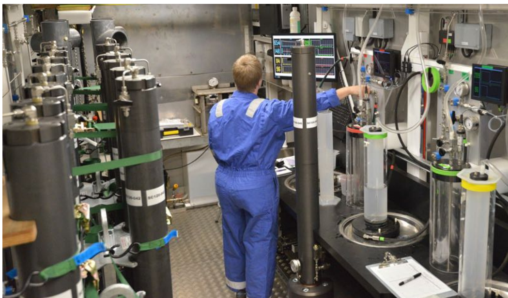
Figure 5. Secure storage and depressurization laboratory for high-throughput quantitative core depressurization.
