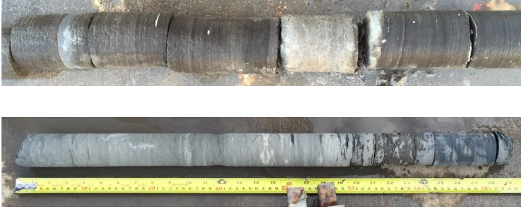
Figure 10. Sections of depressurized core, collected during the 2015 Cameron land test in a hard shale & carbonate formation using both the HPTC (57 mm diameter, upper photo) and the PCTB (51 mm diameter, lower photo) illustrating the effectiveness of these pressure coring systems in harder formations.
