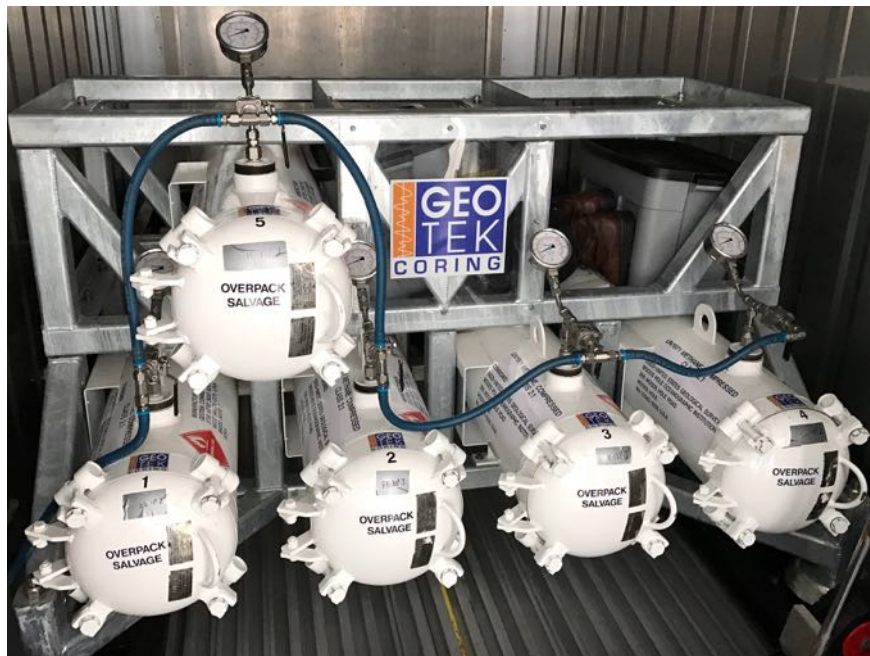
Figure 7. Overpack cylinders containing storage chambers secured and shock mounted inside a specialized refrigerated shipping container.
