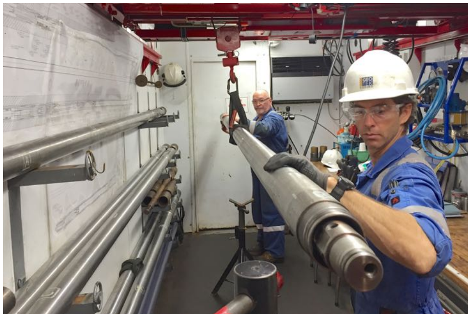
Figure 3. Autoclave section of the PCTB being prepared in the tool service laboratory.
