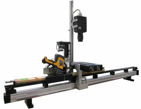
MSCL-XZ with linescan camera, Olympus XRF and point magnetic susceptibility
